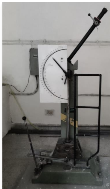
Fig 5: Charpy testing machine
