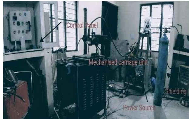
Fig 1: The Welding set-up
