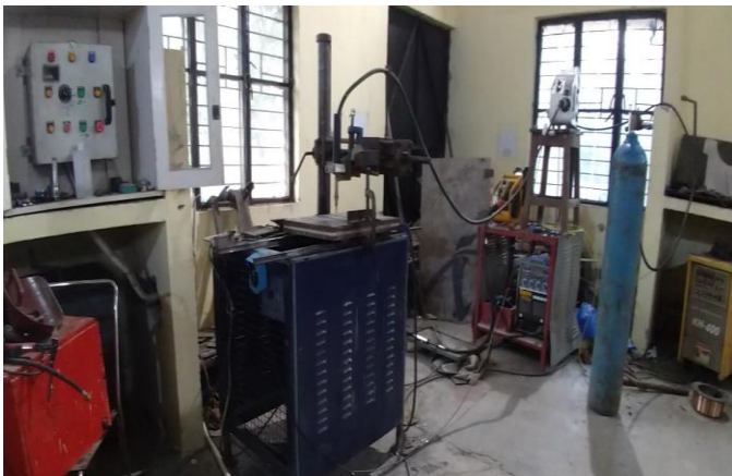
Fig 2: Experimental Setup of MIG Welding
