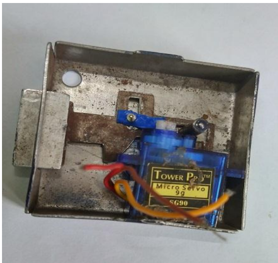
Fig -6: Servo attached to lever.
