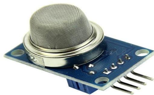
MQ2 measures the smoke, LPG and Corban dioxide. MQ7 measures the Corban monoxide and MQ135 measure the NH<sub>3</sub> (ammonia gas) and No.
