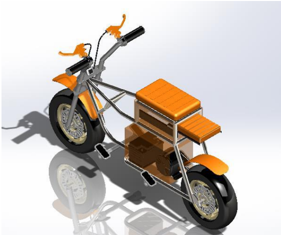
figure 2.2: seat expansion (isometric view)
