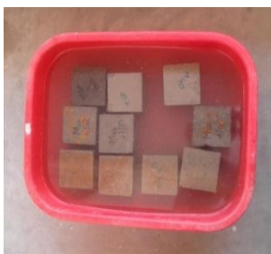
Fig 1 Geopolymer concrete dipped in sulphuric acid
