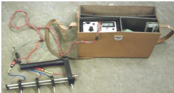
Fig -4: Concrete resistivity measurement – test setup [10]
