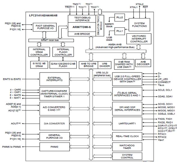
Fig -1: Block diagram of LPC2148
