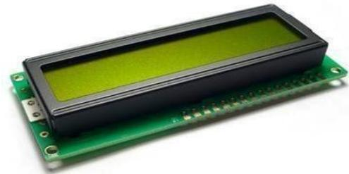
Fig -2: Liquid Crystal Display
