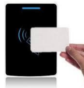
FIG.7. RFID TAG SCANNED USING RFID
