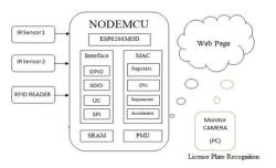
The NODEMCU ESP8266 is an Important part in the parking system.IR sensor would emit and find whether any vehicle is present based on the intensity of the light it received. It then sends the data to NODEMCU ESP8266 where the whole process takes place. The microcontroller Node MCU will make decisions based on data send by the sensor.
