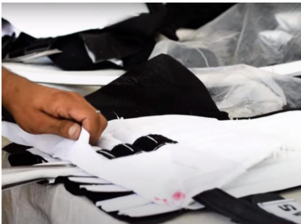
Fig.5 Image of PVC Foam insertion in existing leg guard making.
