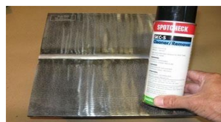
Fig-13: Cleaning the surface
