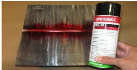
Fig-14: Penetrant application
