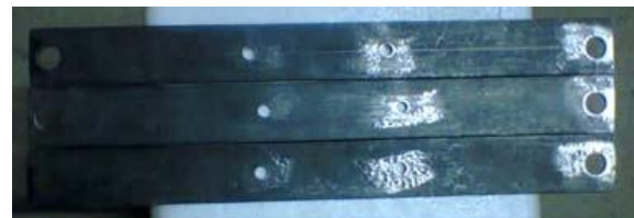
Fig-11: Holes drilled on link
