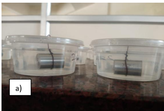
Figure: 3.1 a) experimental set up of corrosion test by immersion technique, b) corrode specimen removed from sea water solution
