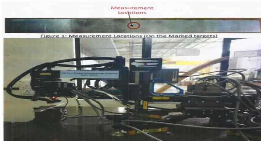
Fig 9: XRD Machine to measure Residual stress
