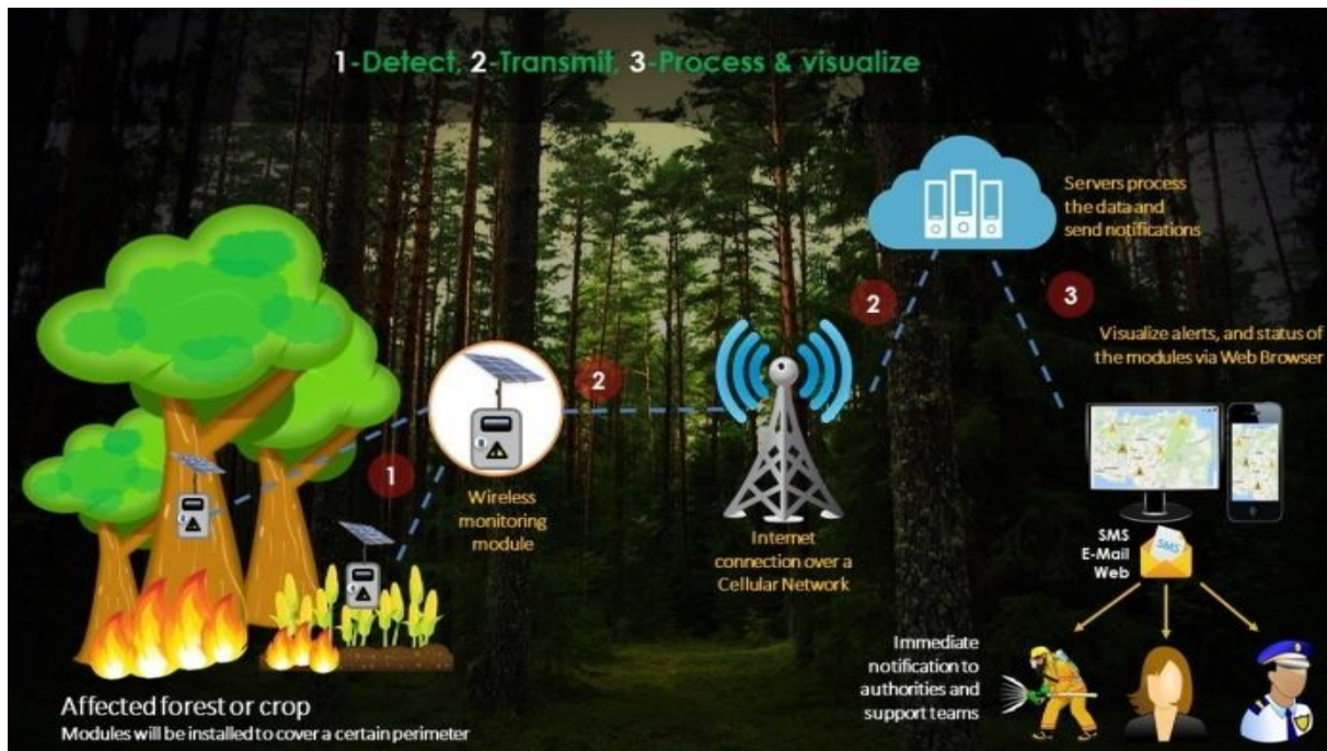
Figure 1. Architecture of fire safety system in a forest or in a crop field using IoT
