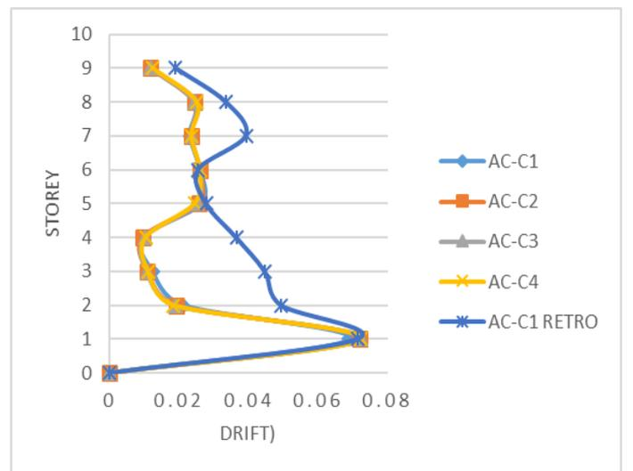
Fig 6: Graph with storey vs drift across the slope
