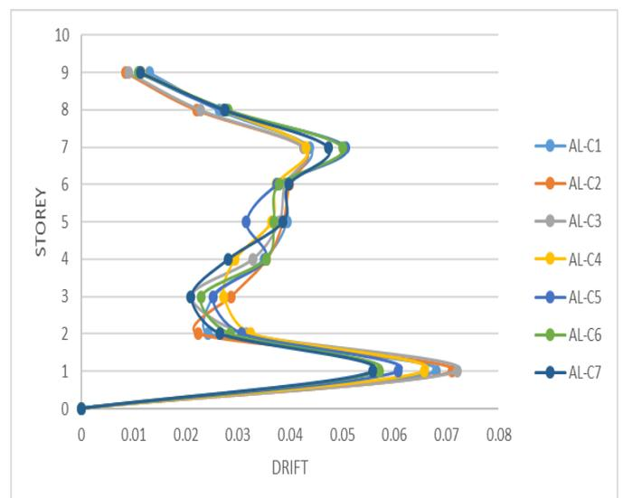
Fig 7: Graph with storey vs drift along the slope
