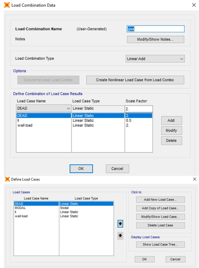
**Fig 4:** linear static analysis in SAP2000
