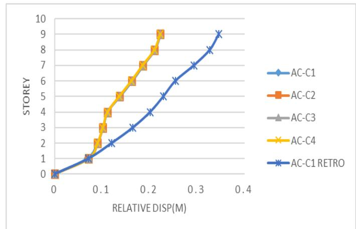
Fig 5: Graph with Storey vs displacement across the slope
