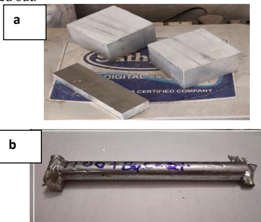
Fig 5.4: a) Aluminum 1100 Ingot and b) Cast Composite
