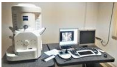
Fig 5.5: ZEISS EVO LS 15kV Scanning Electron Microscope.
