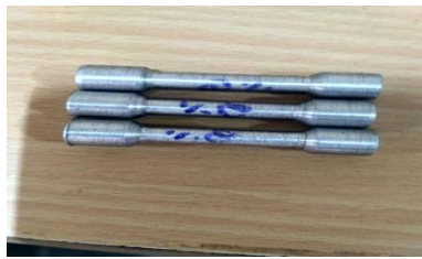
Fig 5.9: Tensile Test specimens as per ASTM standard
