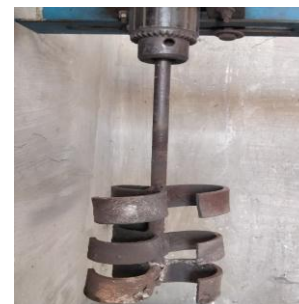
Fig 5.3: Curved radial blade impeller used for the Stir casting
