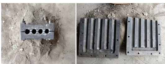
Fig 5.2: Photography showing mould assembly
