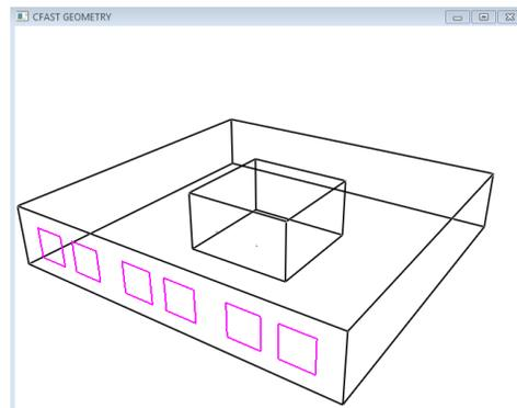
Figure 5: Outline of geometrical structure of warehouse compartments with vents
