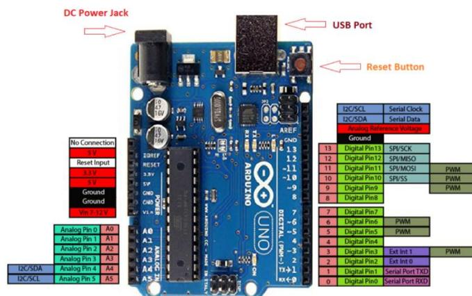
Fig2 Arduino UNO pinout
