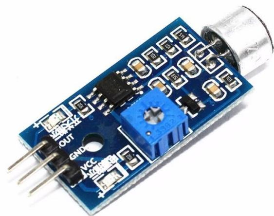
Fig4 LM393 sound sensor module
