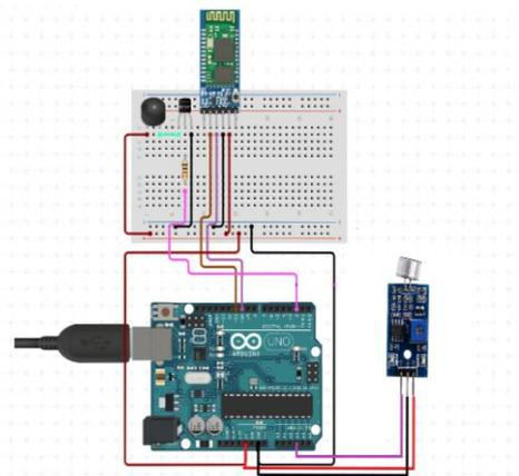
**Fig1 Microcontroller and HC 05 Bluetooth module interface with LM 393 sound sensor module.**
