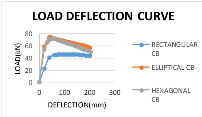
Fig .7 Load Deflection curve comparing three types of opening in doubly webbed castellated beam
