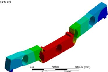
c) Concrete in-filled beam with alternative holes
