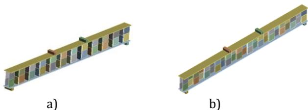
Fig.2 Model of steel strengthened castellated beam by diaphragm placed a)perpendicular b)parallel
