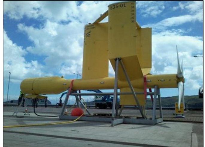
Fig - 4: Tidal Stream Generators
