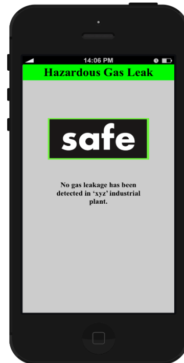
Fig-8: An interface of subscriber application when no gas has been detected.
