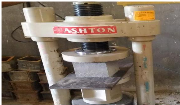
Fig -4: Compressive Strength Test
