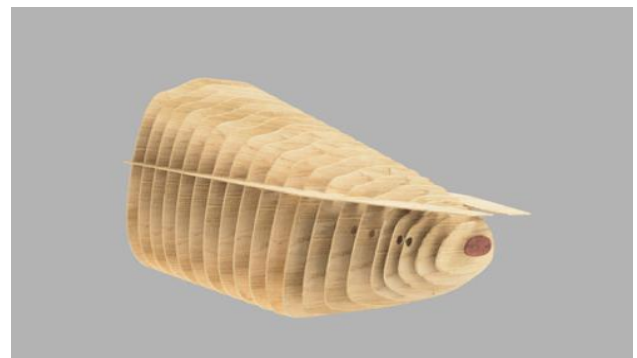
Fig -12: Skeleton made of MDF.
