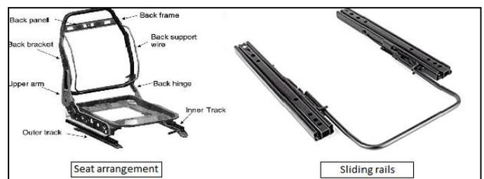
Fig -2.4: Four wheeler seat structure
