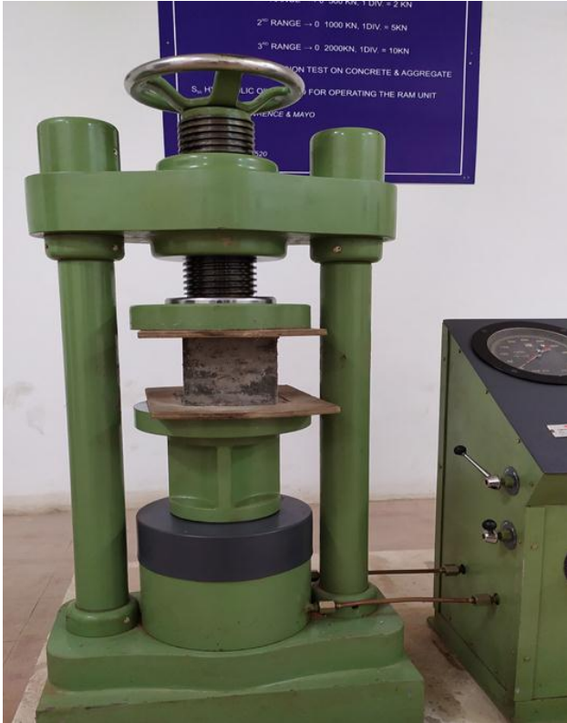
Fig-2: Testing the Cube Specimen
