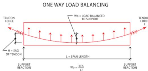
Fig-2: Post tensioning concept
