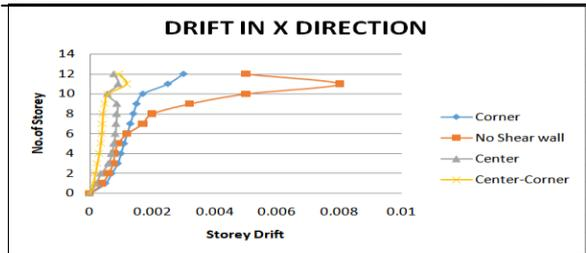
Fig -29: Drift in X-Direction-Model 5
