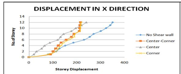
Fig -17: Displacement in X-Direction-Model 3
