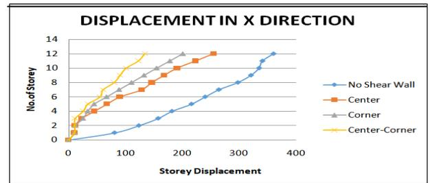
Fig -15: Displacement in X-Direction-Model 2
