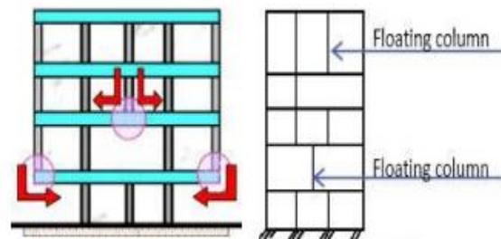
Fig-1: Floating or hanging columns at various positions
