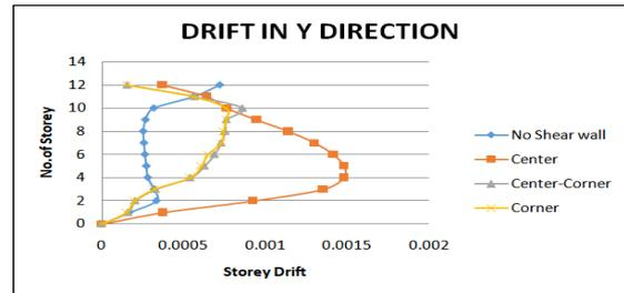
Fig -24: Drift in Y-Direction-Model 2
