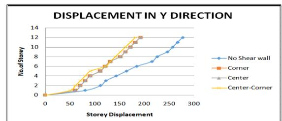
Fig -20: Displacement in Y-Direction-Model 5
