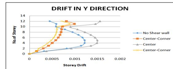
Fig -26: Drift in Y-Direction-Model 3
