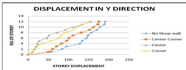
Fig -14: Displacement in Y-Direction-Model 1
