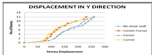
Fig -18: Displacement in Y-Direction-Model 3
