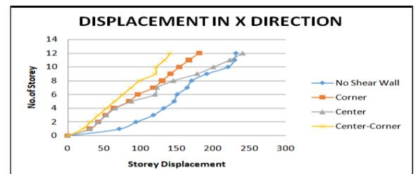
Fig -19: Displacement in X-Direction-Model 4
