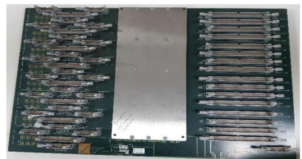
Fig 6. Generic Loadboard of ATE
