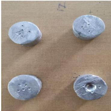
Fig5.6: - Sample Test Piece for Rockwell Hardness Test
