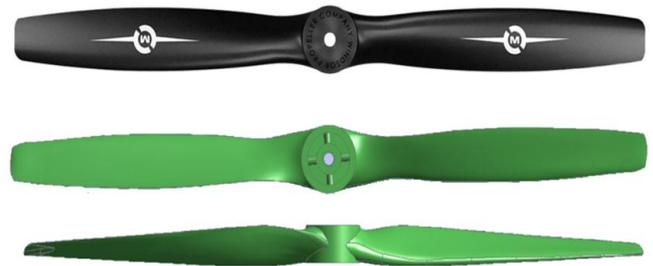
Fig-6: Propeller Scanned views
