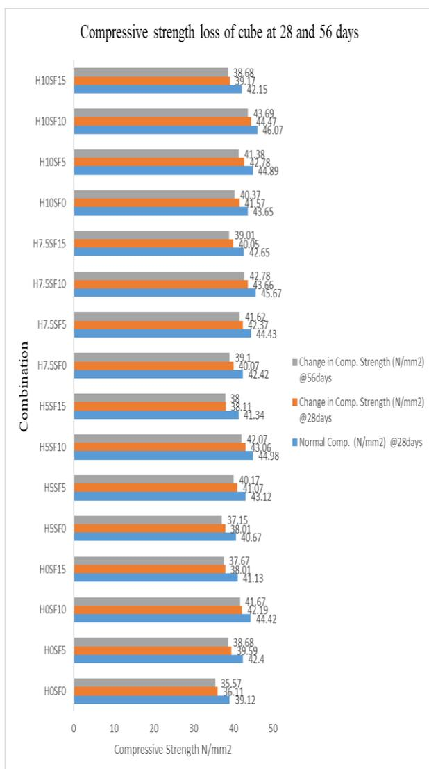
Figure 5 Loss of Compressive Strength N/mm<sup>2</sup> at 28 and 56 days
