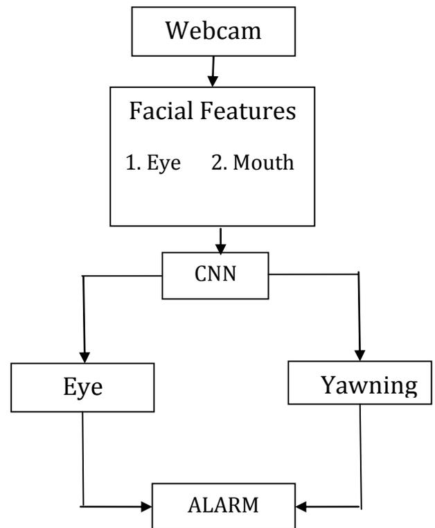
FIG - 1: Architecture diagram of Drowsi Care System
