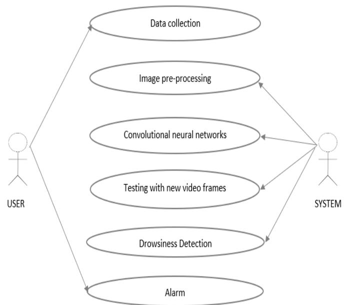
FIG - 2: Use Case diagram of Drowsi Care System.
