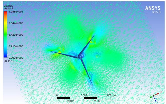
Fig -7: CFD result for 5 m/s wind speed
