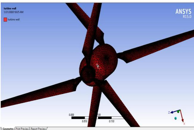
Fig -5: Mesh image of the dual rotor wind turbine
