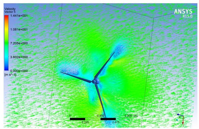
Fig -8: CFD result for 7 m/s wind speed
