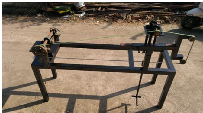
Fig-5: Fabricated Setup for Coating Heat Sealing Belt
