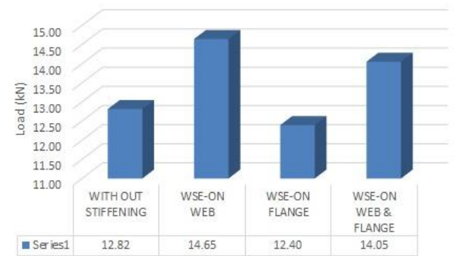
Chart -5: Load comparison graph of models with web openings
