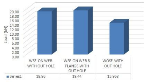
Chart -4: Load comparison graph of models without web openings
