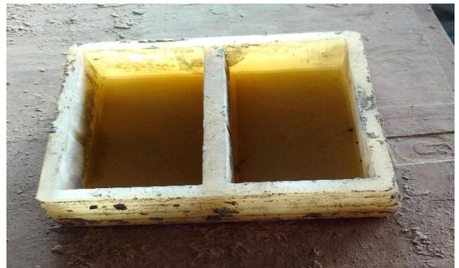
Dry mix containing cement, sand, coarse aggregate was prepared and mixed for about 2 minutes. It was then transferred into molds kept on vibrator machine for minute.
