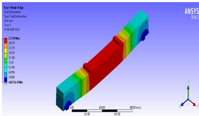
Fig-7: Deflection of Partially encased beam
