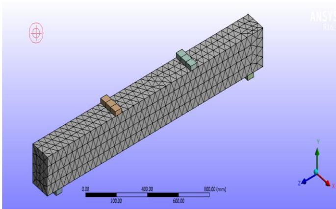
Fig-10: Meshed Partially encased beam
