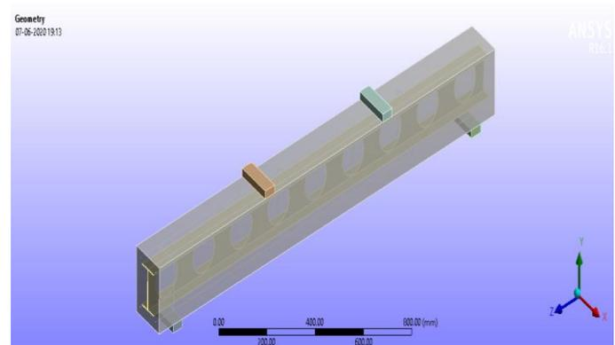
Fig-9: Model of Fully encased beam
