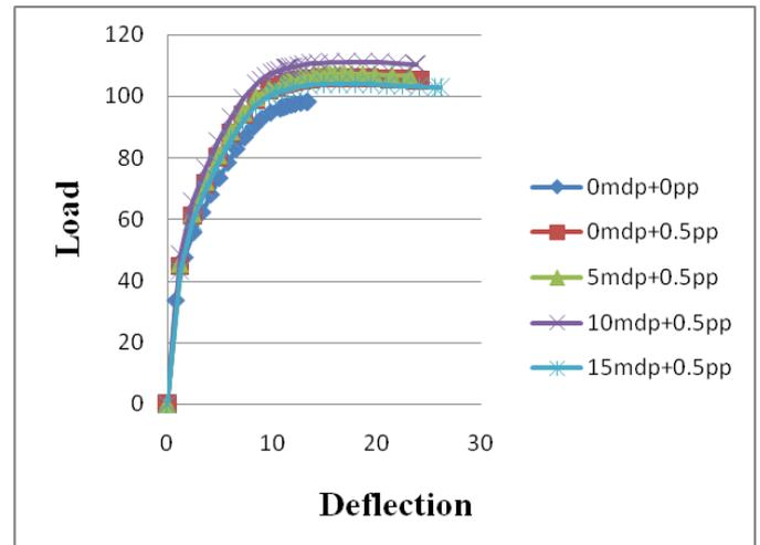
Fig-12: Load-deflection graph of Fully encased beam
