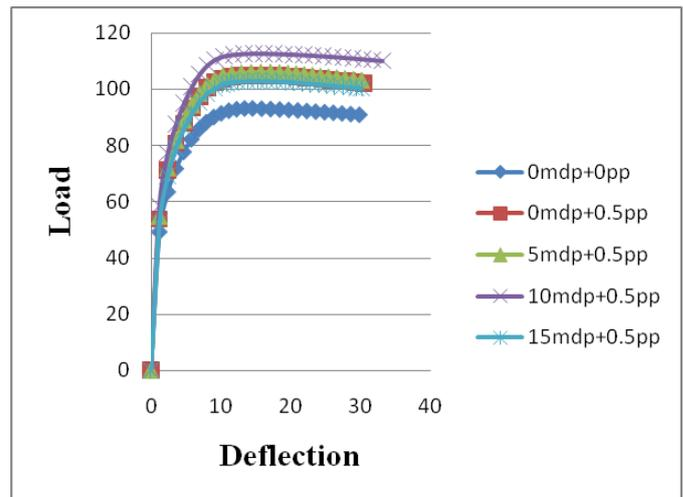
Fig-4: Load-deflection graph of RCC beam
