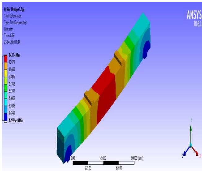
Fig-3: Deflection of RCC beam
