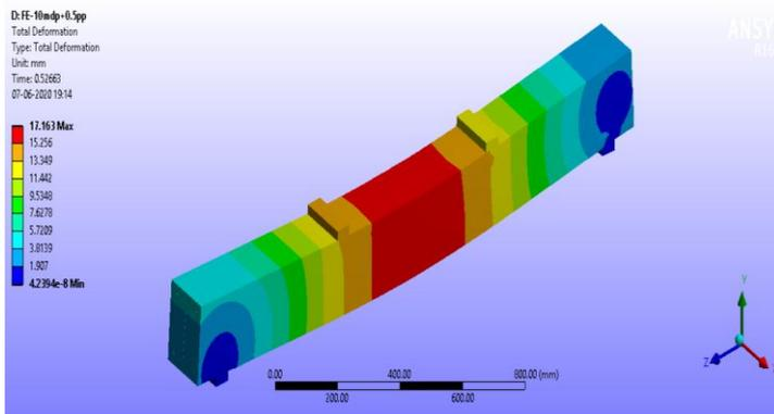
Fig-11: Deflection of Fully encased beam
