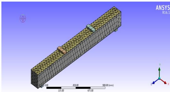
Fig-6: Meshed Partially encased beam
