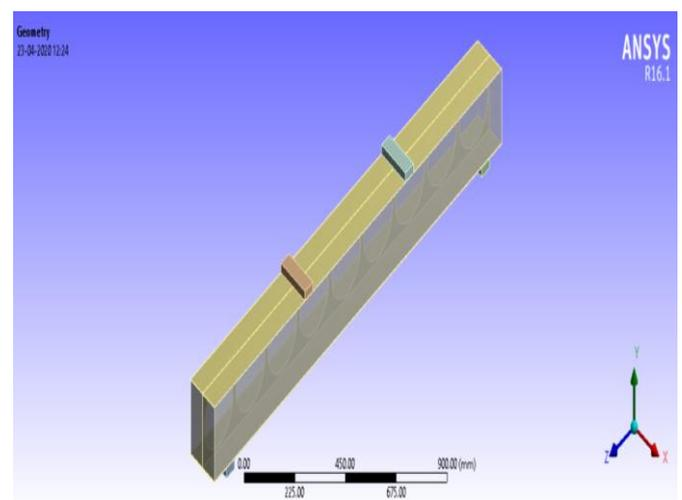
Fig-5: Model of Partially encased beam
