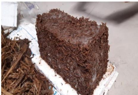
Figure: Mycelium covering brick
