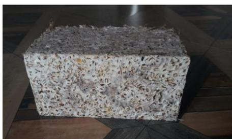
Figure: Mycelium brick
