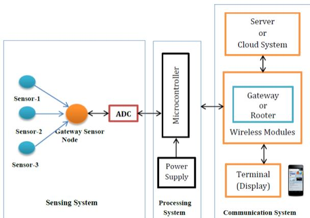
Fig- 3: Typical Architecture of Sensor Node
