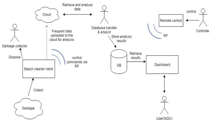
**Fig -1: Top level flow diagram**
