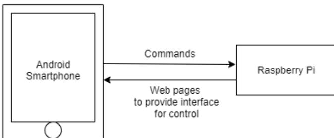
Fig -9: Interfacing the bot with an android smartphone.
