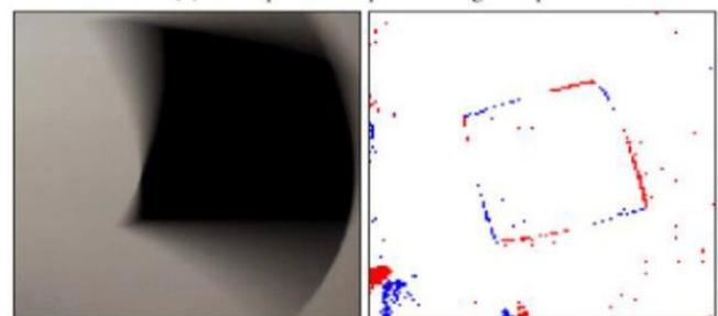
(b) Standard CMOS camera (c) Integrated DVS events (2 ms)
