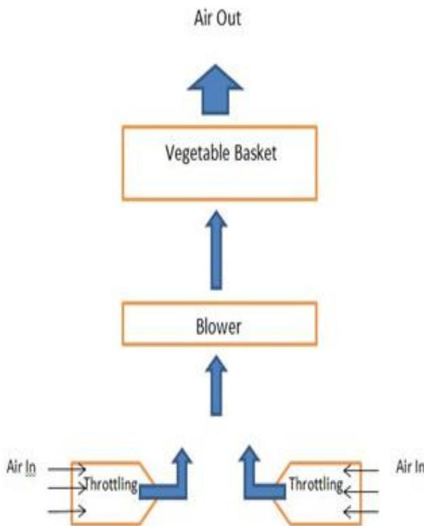
Fig.-3: Flow diagram shows throttling process
