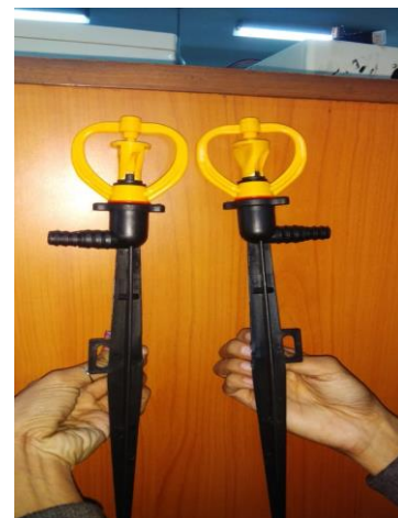
Fig -5: Irrigation sprinklers
