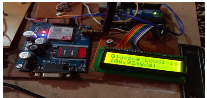
Fig -3: Hardware model of GSM based needleless blood glucose monitoring system.
