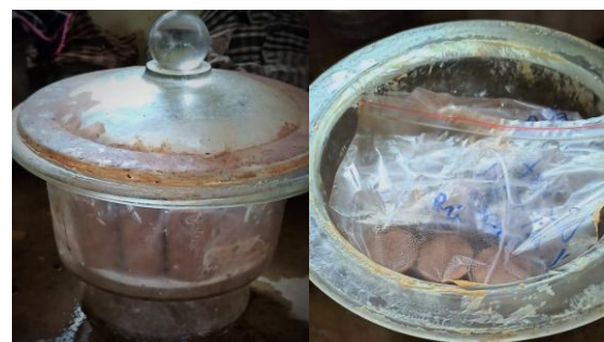
Fig -4: Curing of Soil Samples in Desiccators
