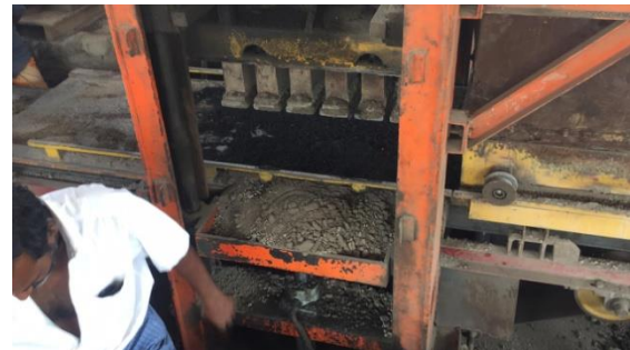
Fig -1: Compaction of brick by machineries
