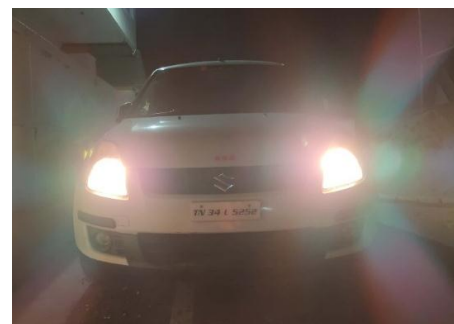
Fig -2: Difference in the glare caused between both headlamps by the use of translucent material
