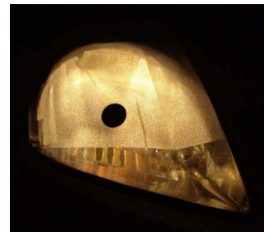
Fig -1: Equivalent translucent material adhered to the left side front headlamp
