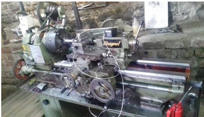
Fig 4.1 Setup for temperature measurement using thermocouple on lathe machine
