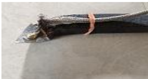
Fig 4.3 Cutting tool with thermocouple inserted
