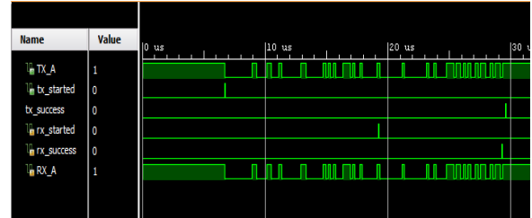
Fig. 10: Frame transmission and reception
