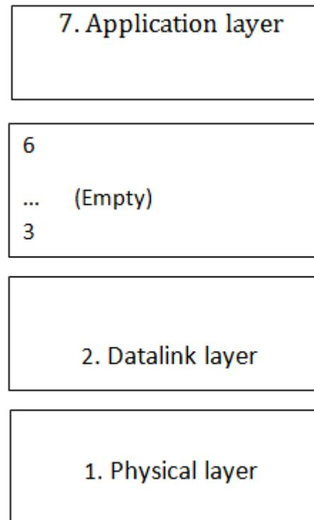
Figure 2. The hierarchical structure of CAN bus
